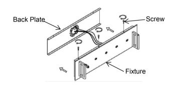
Attach fixture to the back plate, using screws provided.
