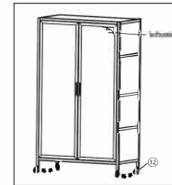
Install casters: Screw the casters into the threaded pipe at the bottom of the side frame. Attention: During installation, support the cabinet to prevent tipping. Finally, remove the protective film from the cabinet door to complete the installation.
