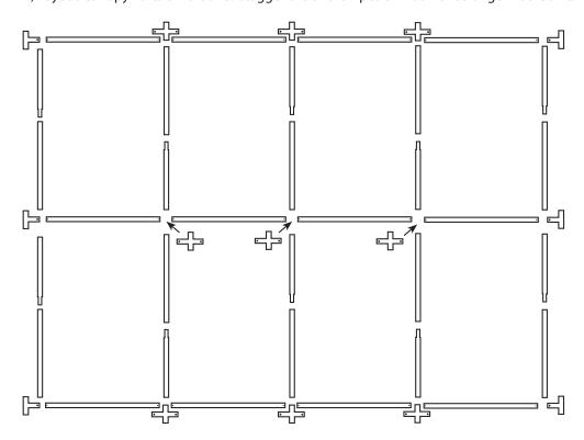
2) Assemble Frame Starting with Center Ridge.
