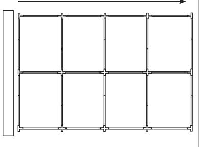
4) Secure the 4 Corners from Underneath with the Corner Straps Sewn in the Corners. Slip a C-Clip on to each the Legs. Lift one Side of the Canopy and Attach the Legs and Foot Pads. Starting with the Center Legs. Attach 10 Ball Bungee Cords located on Underside of Cover to the Frame.
