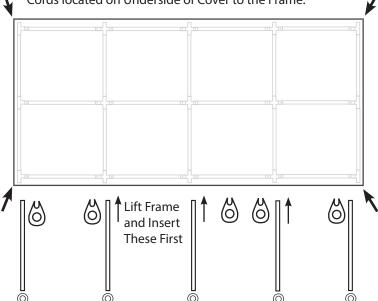
5) Lift the Opposite Side of the Canopy and Attach the Legs and Foot Pads in Same Way. Begin with the Center Legs.
