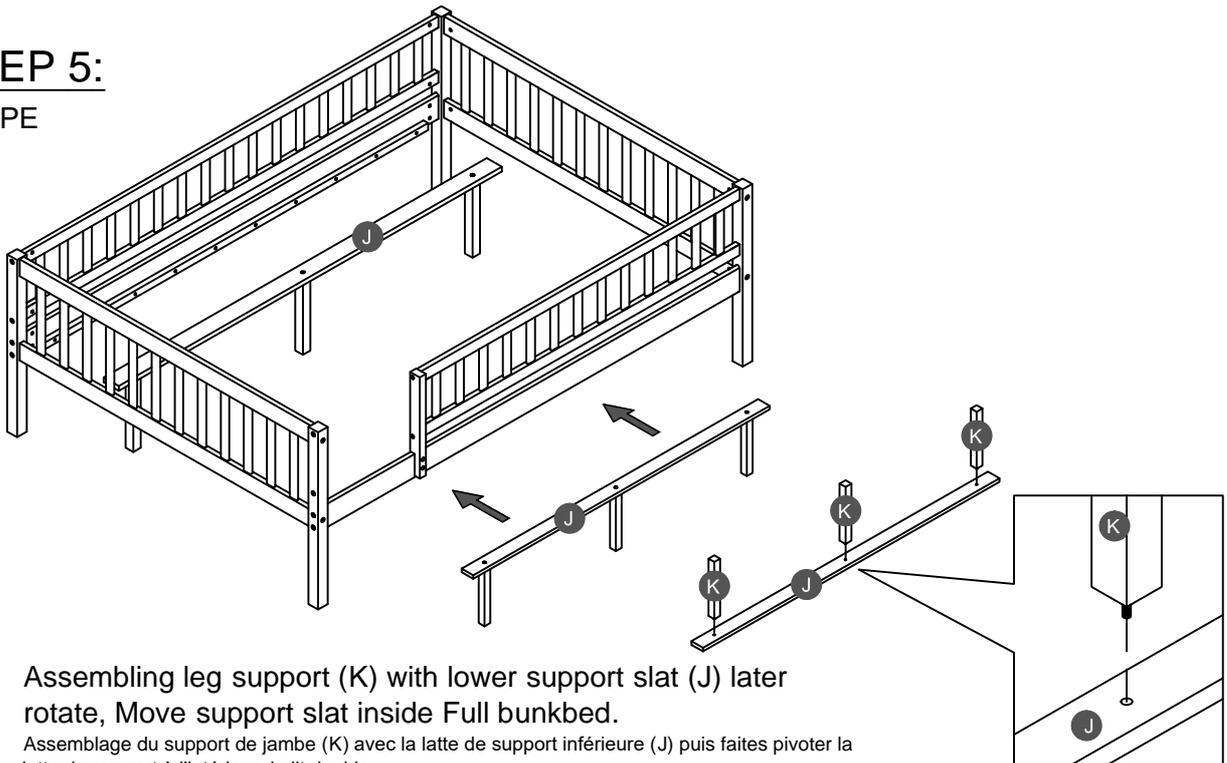
Assembling leg support (K) with lower support slat (J) later rotate, Move support slat inside Full bunkbed.
