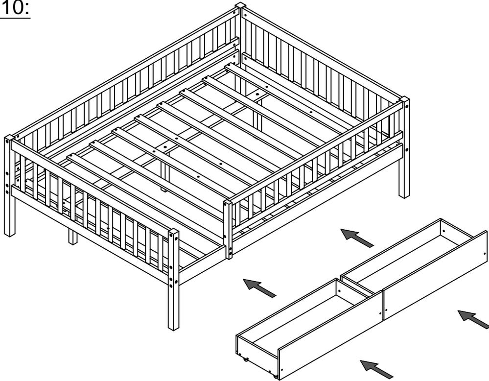
Push Drawer under the bottom of Bunkbed.
