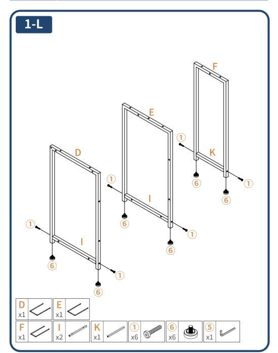
The direction of the screw holes pointed by the arrow on E and F should face outward when assembling.
