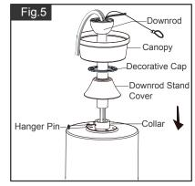
Loosen the collar screws out part way. Insert the downrod into the collar. Slide hanger pin through holes of collar and downrod.
