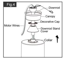
Thread the motor wires through the downrod stand cover, decorative cap (Making sure the smooth side of decorative cap is facing downward.), canopy and downrod.
