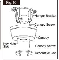
Remove one canopy screw (for later use), then push the canopy upwards by inserting canopy screw head left in hanger bracket into key hole slot, rotate the canopy till the hole in canopy aligns the hole in hanger bracket, finally, secure the canopy to hanger bracket with
