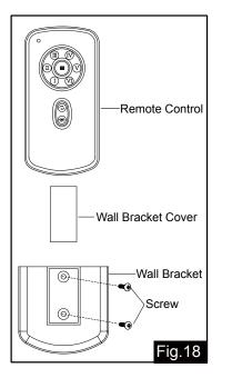
Slide off the wall bracket cover from the wall bracket. Install the wall bracket on a wall with the two screws included. Place the wall bracket cover back on the wall bracket to cover the screws. Slide the remote control into the wall bracket.
