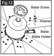
Thread the blade screws through the washer, blade into blade holder. Tighten all blade screws securely. Repeat to other blades. **Note: Alternate long blade** with short blade to keep balance.
