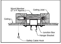
Tighten the hanger bracket to the outlet box with two mounting screws. (Make sure the outlet box is securely installed so that it will be able to support at least the fan weight.) Attach the safety cable hook to the ceiling and make sure the safety cable hook is covered by the fan canopy.
