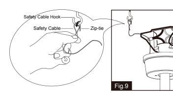
Hang the safety cable into the safety cable hook, tighten the safety cable to the safety cable hook by using the zip-tie.
