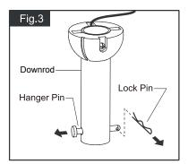
Remove the lock pin from the hanger pin and remove the hanger pin from the downrod.
