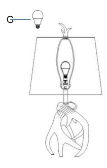
Step 2 Insert the bulb(G) into the socket(C).
