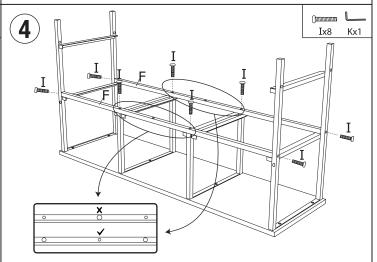
**Step 4:** Position the frame poles (F) into place and secure with screws (I) as shown. Make sure the holes are facing the right direction. Follow key above.
