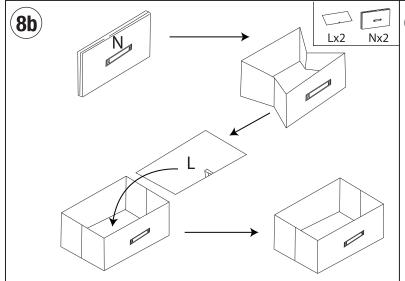
Step 8b: Unfold drawers (N), then place inset pad (L) inside.
