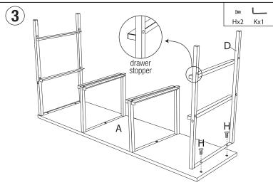
**Step 3:** Secure frame (D) to wood top (A) as shown above with screws (H) then secure with wrench (K). Please make sure the holes of the drawer top and the frame match the picture above. The drawer stopper should be facing the back.
