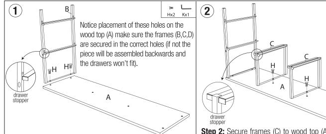
**Step 1:** Secure frame (B) to wood top (A) as shown above with screws (H) then secure with wrench (K). The drawer stopper should be facing the back.
