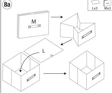
Step 8a: Unfold drawers (M), then place inset pad (L) inside.
