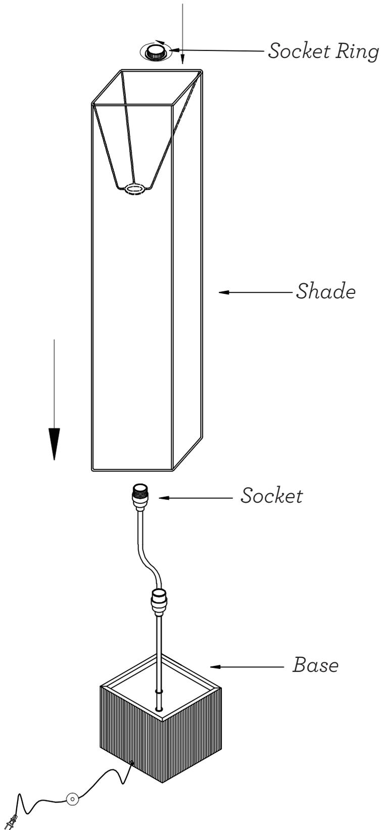
1. Set shade onto socket and tighten clockwise with socket ring.
