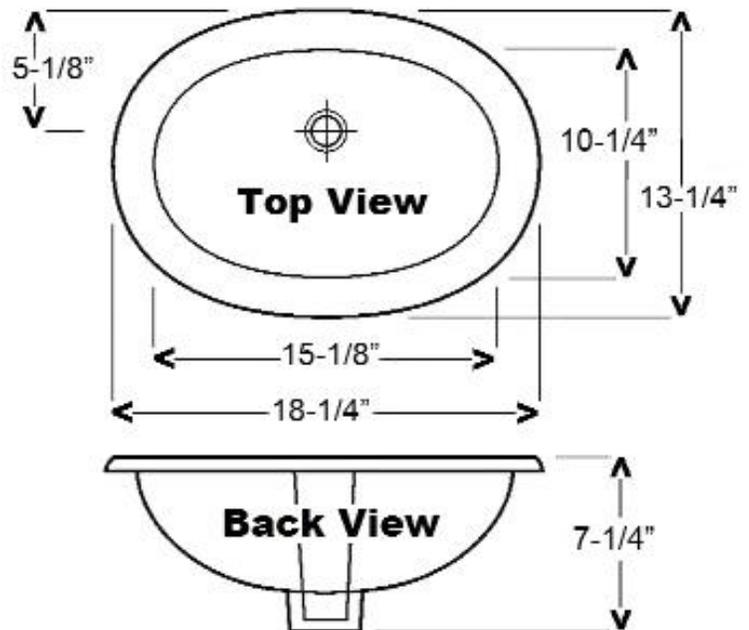
Dimensions of fixture are nominal and may vary within the range of tolerances established by ASME Standard A112.19.2.2013. Dimensions and specifications subject to change without notice.
