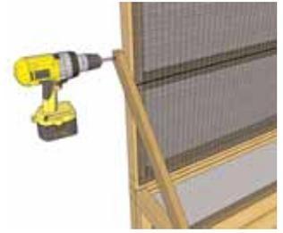
**7.** To install **Trellis/Lid Arms (C)**, measure **16"** up from **bottom** and **17"** from the **rear of panel**. Pre-drill shallow **1/8"** hole **3/8"** from top of framing to help you position arm. Locate **Trellis/Lid Arm Spacer** and position next to framing. Screw top of arm to **Trellis/Lid panel** with **1 - 2"** screw. Do not overtighten.
