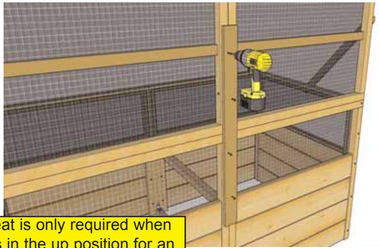
**Note;** Rear Trellis Cleat (D) is only required when you plan to use Trellis in the up position for an extended period of time. Not required if you plan on opening and closing your lid often.
