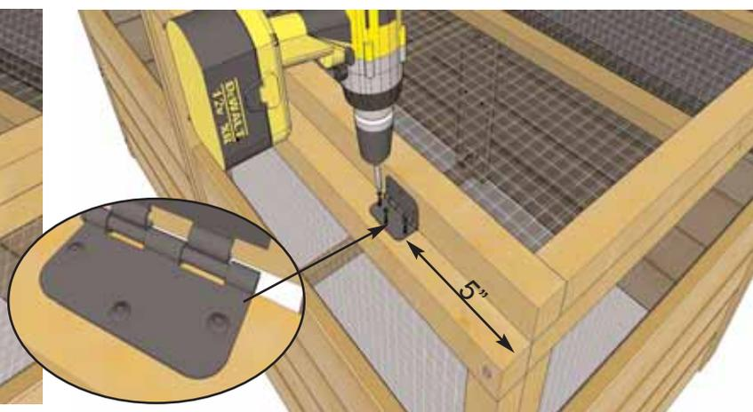
**4.** With Trellis/Lid evenly positioned on raised bed framing, locate **4 Black Plastic Hinges - Part B** and **24 - 3/4" Black Screws**. Align 1st hinge with counter sunk holes facing up. Position hinge approx. 5" from end. Attach to top framing of 6x3 raised bed with **3 - 3/4" Black Screws** per hinge. Pre-drill shallow hinge holes first with 1/8" drill bit to prevent wood from splitting. Do not over screw with cordless screw gun!
