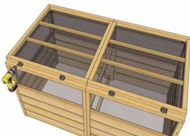
**5.** Complete attachment of 1st hinge by screwing **3 - 3/4" Black Screws** into the lid framing as shown above. Evenly space remaining hinges and attach as described previously.
