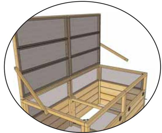
**8.** At the bottom of arm, attach a **2"** screw to a **1"** depth in previously marked location. Arm notch will rest on screw and prevent **Trellis/Lid** from closing.
