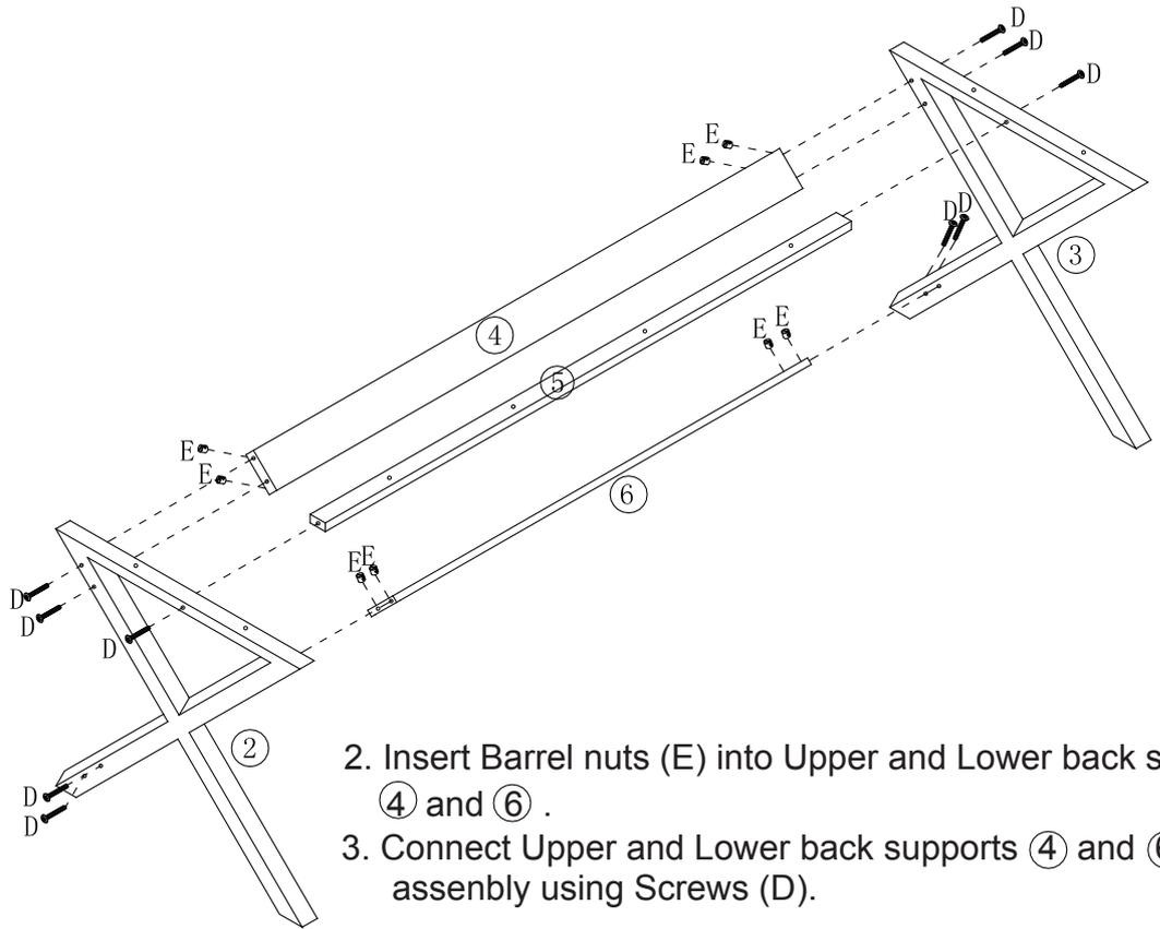
2. Insert Barrel nuts (E) into Upper and Lower back supports (4) and (6) .
