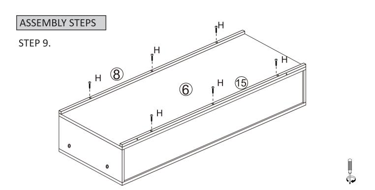
Fix parts (8), (15) to the bottom panel (6) using 6 x screws (H) with a screwdriver.
