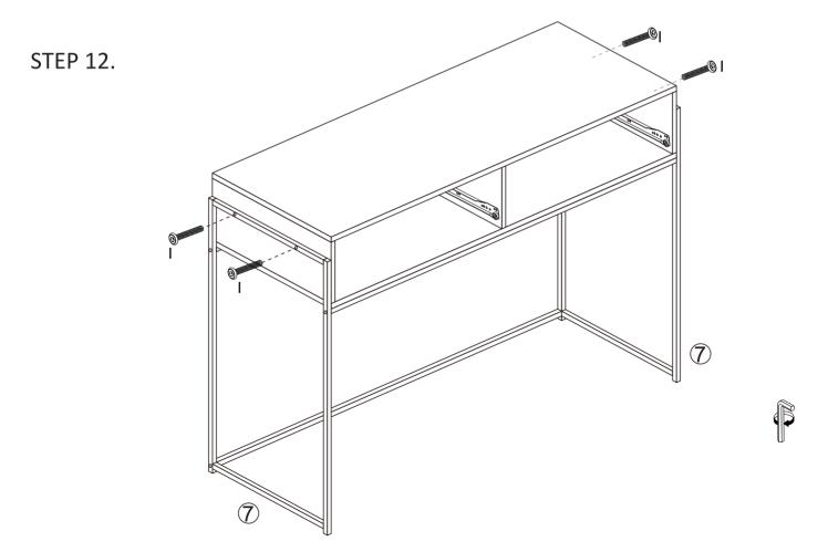
Insert and secure 4 x bolts (I) into position as shown to lock it. Tighten with Hex key.
