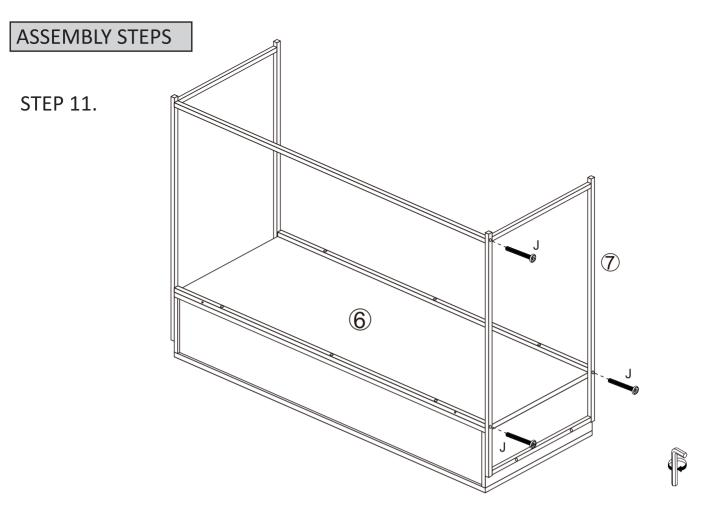
Attach the other piece of metal frame (7) to assembled unit using  $3 \times 10^{-5} \times 10^{$
