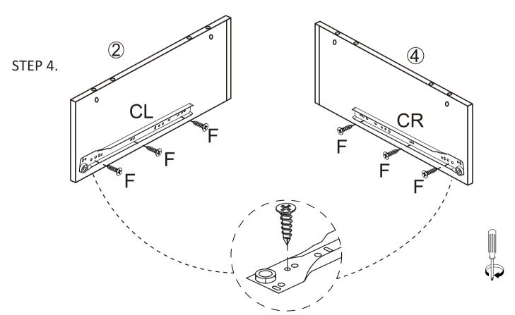
Attach 2 x rails (CL), (CR) to panels (2), (4) using 6 x screws (F) as shown. Tighten with a screwdriver.
