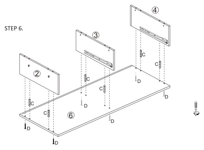
Attach panels (2), (3) and (4) to panel (6) using 6 x wooden dowels and 6 x screws (D) as per diagram. Tighten with a screwdriver.
