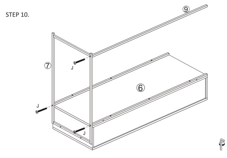
Attach metal frame (7) and metal beam (9) to assembled unit using  $3 \times 10^{-2} \times 10^{$
