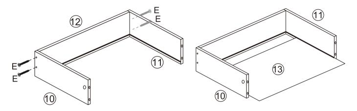
Attach panel (10), (11) to panel (12) using 4 x screws (E). Tighten with a screwdriver.
