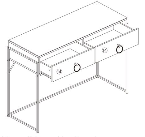
Slide assembled drawers into position as shown. Final assembly.
