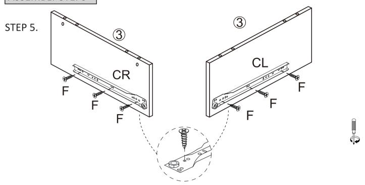
Attach 2 x rails (CR), (CL) to panel (3) using 6 x screws (F) as shown. Tighten with a screwdriver.
