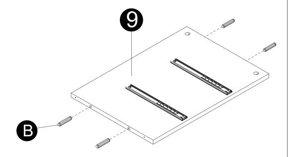
· Insert dowels (B) into panels (7,9).
