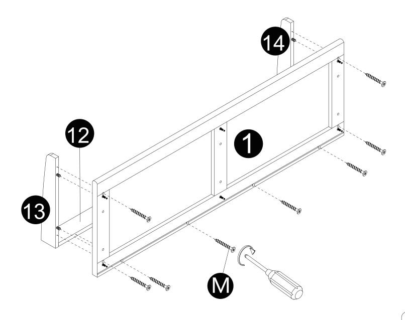
· Attach panels (12,13,14) to panel (1) with screws (M) correctly.
