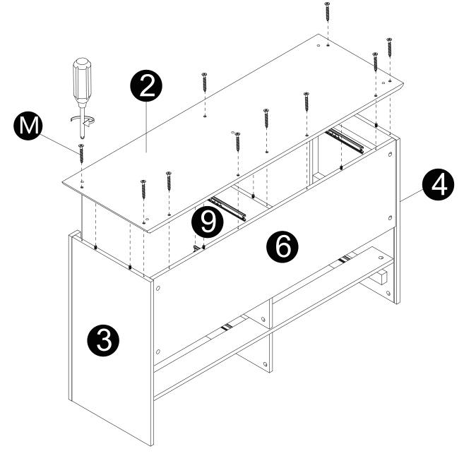
· Attach panel (2) to panels (3,4,6,9) with screws (M) correctly.
