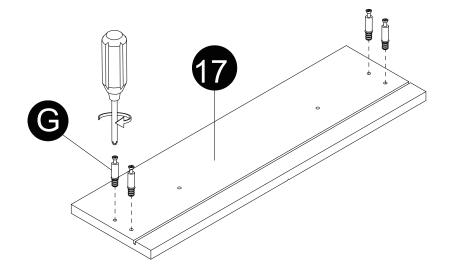
· Screw cam bolts (G) into panels (16,17).
