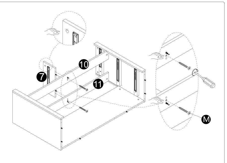
· Attach panel (7) to panels (10,11) with screws (M) correctly.
