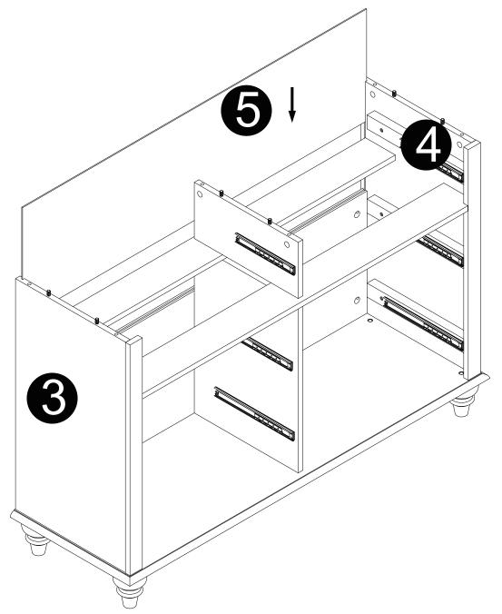
Carefully slide panel (5) into place along the back of the assembly.
