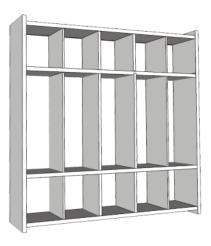
Step 14: Finish tightening all hex screws. DO NOT OVER TIGHTEN. DO NOT DRILL. Stand unit upright so that it it is resting on bottom piece and the edges of Side A and B. Assembly is complete.
