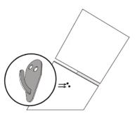
**Step 1:** Attach hooks to divider pieces by using Phillip's head screwdriver to screw small screws into pre-drilled holes before assembling unit. Make sure hooks are pointed upwards toward the shortest end of the divider panel as seen in illustration.
