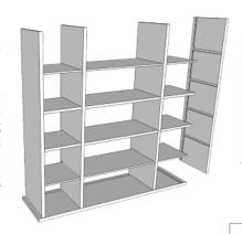
Step 9: Insert edge of top piece into remaining mortise of Side A aligning back grooves. Insert edges of each divider into the corresponding mortise on top piece. Insert hex screws into (4) pre-drilled holes of top piece and tighten down half way. DO NOT DRILL.
