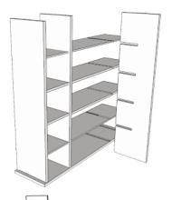
Step 8: Insert top shelf parallel to bottom shelf, fitting the grooves of top shelf into remaining grooves of dividers. Make sure back grooves are aligned. Edge of shelf should be inserted into remaining mortise of Side A. Insert hex screws into (2) pre-drilled holes in Side A and tighten down half way. DO NOT DRILL.
