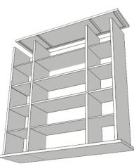
Step 13: Fit Side B over edges of the assembled pieces, inserting edges of bottom piece, bottom shelf, top shelf and top piece into mortises of Side B. Make sure that back panels fit into back grooves of Side B. Insert hex screws into each of (8) pre-drilled holes on Side B and tighten down half way. DO NOT DRILL.
