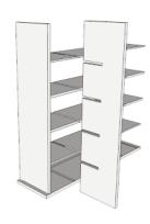
Step 7: Insert bottom shelf parallel to bottom piece, fitting the grooves of bottom shelf into grooves of dividers. Make sure back grooves are aligned. Edge of shelf should be inserted into mortise of Side A. Insert hex screws into (2) pre-drilled holes in Side A and tighten down half way. DO NOT DRILL.
