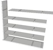
Step 6: Insert edge of final 3/8" divider (end without hook) into remaining mortise of bottom piece. Make sure that notches of divider face away from back grooves of bottom and Side A. DO NOT DRILL.
