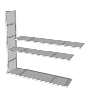
**Step 4:** Insert edge of other 5/8" divider (end without hook) into second center mortise of **bottom** piece. Make sure that the notches of divider face away from back grooves of **bottom** and **Side A.** Place a hex screw in each of (2) pre-drilled holes in **bottom** piece and tighten down half way. DO NOT DRILL.
