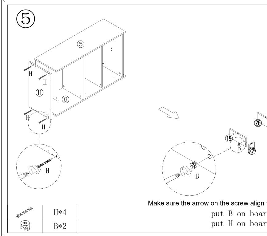
Make sure the arrow on the screw align to the hole on the side.
