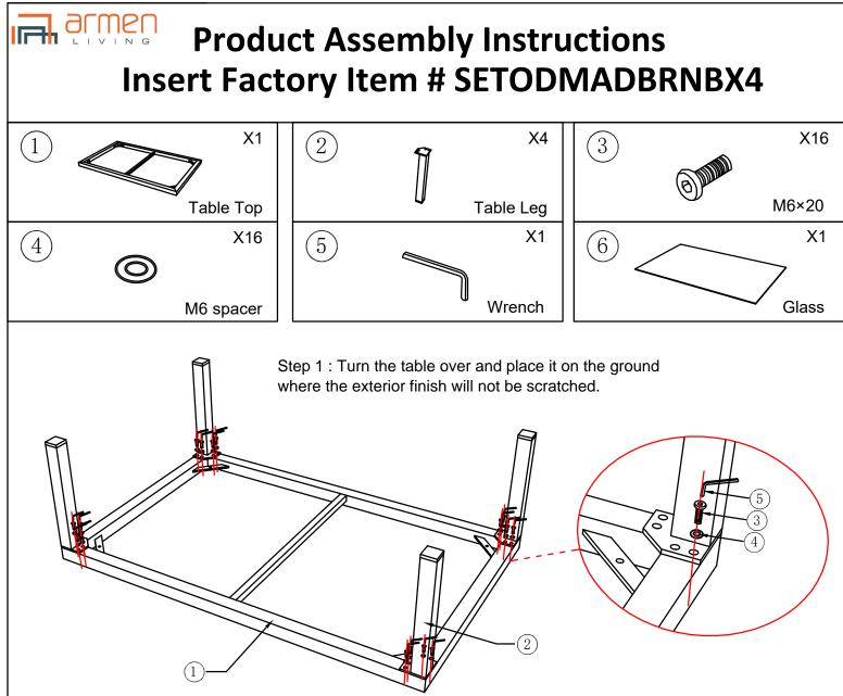
Step 2 : Align the screw holes of the table legs with the screw holes of the table top, insert flat washers(4) and screws(3) into each hole, once the screws are in place, tighten the screw until firmly attached with the wrench provided.
