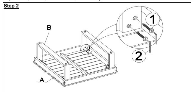
Place the Table top (A) facedown on a clean, non-marring surface as shown above Attach the Leg (B) to the Table top (A) by using Bolts (1) and Allen Key (2). Repeat the same process with the remain Leg (B)
