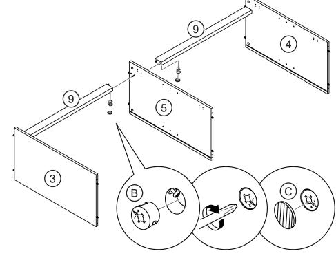
Assemble the left panel (3), medial panel (5), right panel (4), and back supports (7) to the bottom panel (2).
