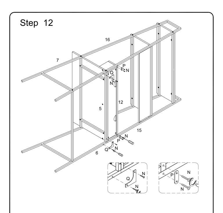
Attach plate (P) and corner plate (Q) to part (12,5) using screw (N) with screwdriver.
