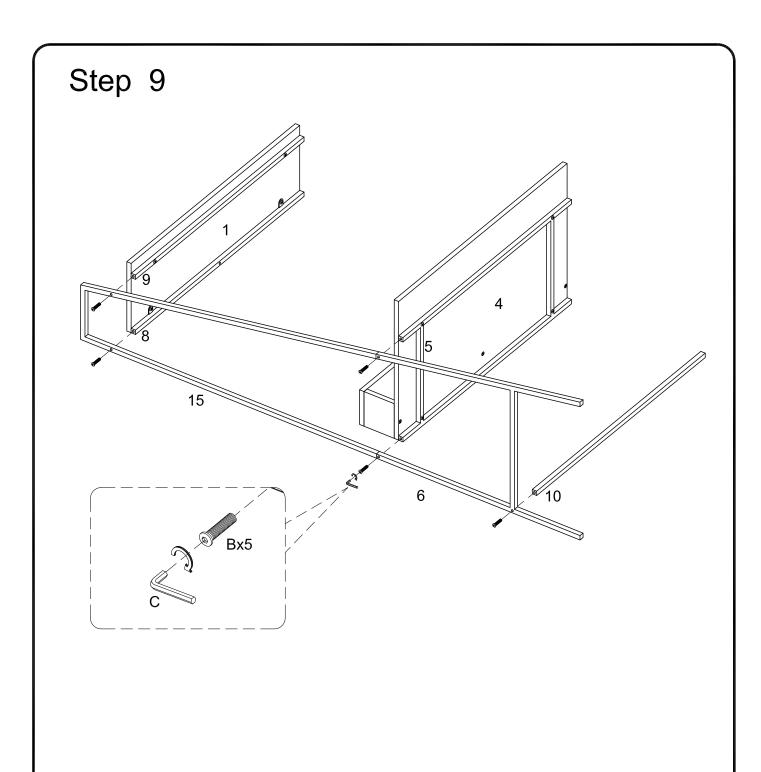
Attach part (15,6) to part (1,9,8), part (5,4), part 10 using bolt (B) with hex key (C).
