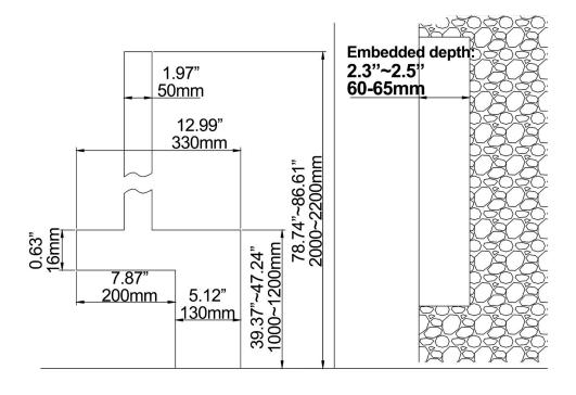
2. Install the main body, water inlet and outlet pipes.
