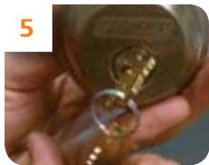
**5** Rotate the key to the two o'clock position.
