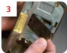
**3** Open built-in door on exterior portion of keypad lock.
