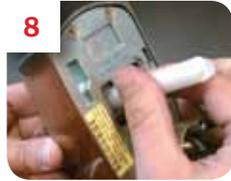
**8** Use follower bar to slide keypad lock housing away from cylinder. Do not remove follower bar. !
