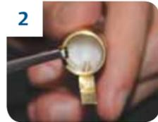
**2** Install spring into back chamber and balance top pin (#3) on top of spring.
