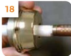
18 Push cylinder back into cylinder housing using the follower bar. **Remove the key.**
