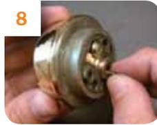
8 Remove spring behind cylinder pin.
