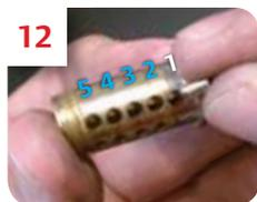
**12** Insert correct numbered pin into first hole, reading cylinder right to left. !
