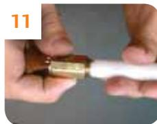
11 Use follower bar to slide cylinder housing away from cylinder. Do not remove follower bar. !
