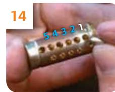
14 Insert correct numbered pin into first hole, reading cylinder right to left. !
