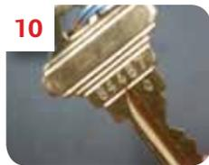
**10** Locate key cut number on new key. Insert new key into cylinder. \*
