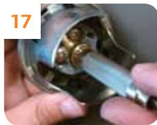
17 Use cylinder cap removal tool to tighten cylinder cap back on cylinder.
