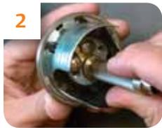
**2** Use cylinder cap removal tool to remove cylinder cap.
