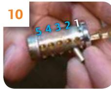
**10** Insert correct numbered pin into first hole, reading cylinder right to left. !
