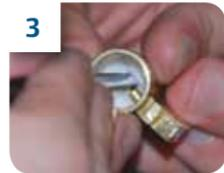
**3** Using follower bar groove as a guide, push pin into its chamber against spring pressure with flat edge of tweezers or small flat blade screwdriver.
