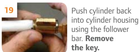
Push cylinder back into cylinder housing using the follower bar. **Remove the key.**
