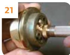
21 Use cylinder cap removal tool to tighten cylinder cap back on cylinder.
