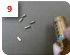
**9** Empty existing pins out of cylinder. **Remove original key.**
