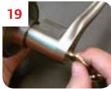
Insert new key and rotate until you can lock the lever component in place.
