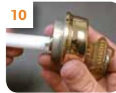
10 Use follower bar to slide cylinder housing away from cylinder. Do not remove follower bar. !
