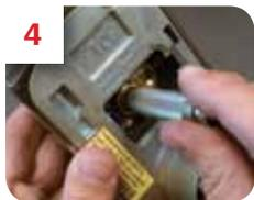
**4** Use cylinder cap removal tool to remove cylinder cap.
