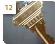
12 Locate key cut number on new key. Insert new key into cylinder. \*
