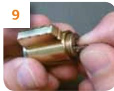
9 Remove spring behind cylinder pin.
