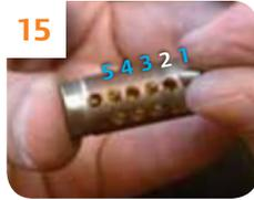
15 Insert correct numbered pin into second hole.
