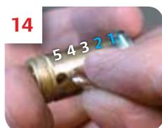
**14** Insert correct numbered pin into third, fourth and fifth holes.
