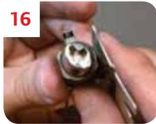
Insert C clip back on cylinder. **Remove the key.**
