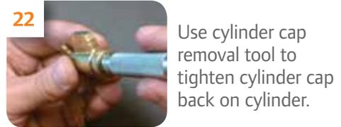
Use cylinder cap removal tool to tighten cylinder cap back on cylinder.
