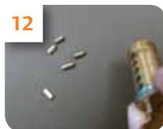
12 Empty existing bottom pins out of cylinder. **Remove original key.**
