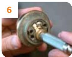
6 Use cylinder cap removal tool to remove cylinder cap.
