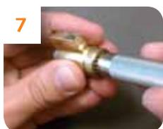
7 Use cylinder cap removal tool to remove cylinder cap.
