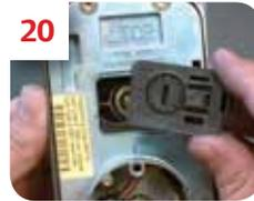
**20** Replace built-in door back onto lock assembly.
