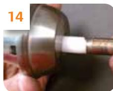
**14** Push cylinder back into deadbolt housing using the follower bar. **Remove the key.**
