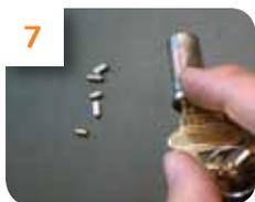
**7** Empty existing bottom pins out of cylinder. **Remove original key.**
