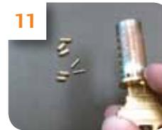
11 Empty existing bottom pins out of cylinder. **Remove original key.**
