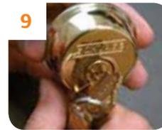
9 Insert original key and rotate it to the two o'clock position.
