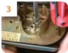
3 Remove the six screws from exterior portion of keypad deadbolt. !
