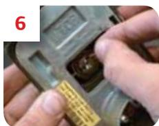
**6** Remove spring behind cylinder pin.
