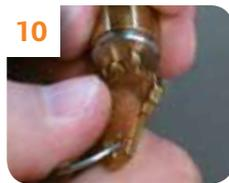
10 Insert original key and rotate it to the two o'clock position.
