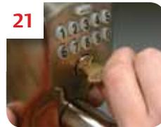
**21** Simulate locking and unlocking the keypad lock to confirm rekey success.
