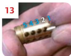
**13** Insert correct numbered pin into second hole.
