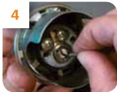
**4** Remove spring behind cylinder pin.
