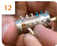
**12** Insert correct numbered pin into third, fourth and fifth holes.
