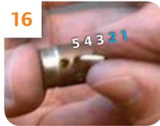
16 Insert correct numbered pin into third, fourth and fifth holes.
