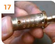
17 Verify all inserted pins are completely flush with top of cylinder. \*
