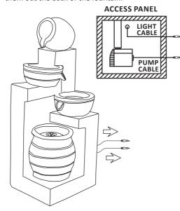
**3.** Fill the reservoir with water, ensuring the pump is completely submerged during operation; approximately 2 gallons.
