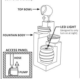
**2.** From the access panel in the back of the fountain, locate the hose and light cables. Attach the pump to the hose and place it inside the fountain.
