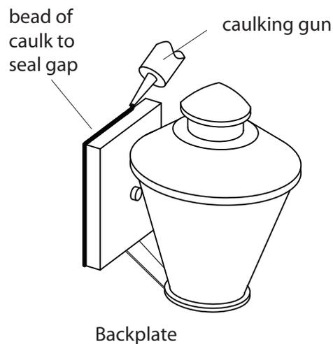
1. After securing fixture in place it is recommended that the gap between the mounting top and fixture base be sealed with any good quality waterproof caulk or silicone sealant. (NOT INCLUDED). It is also recommended that a small bead of caulk or sealant be put under the ball knobs used to mount fixture. See Drawing 2.
