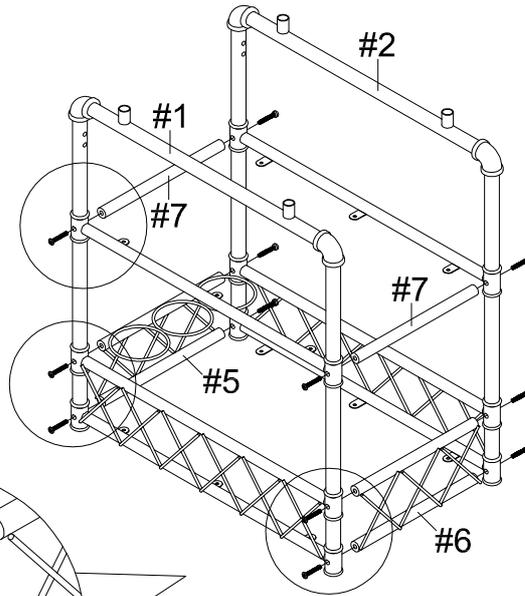
1) Align rear lower frame (#5) to the left and right frame (#1,#2). Secure with bolts (#B) by using the Allen wrench (#E).
