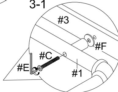
1) Align the top (#3) to the top of the frames. Make
