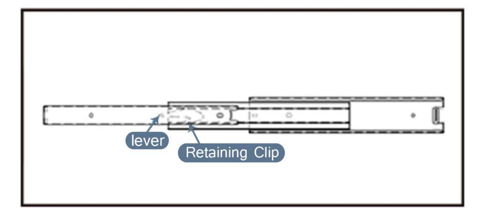
down the left slide. Pull the drawer completely and take it out. To reinstall the drawer, replace it on its slides and push it completely.
