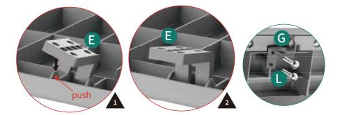
For easier installation, part E should tilt to the one side, then to the other.
