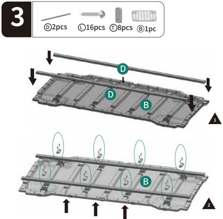
Slightly lift panel B to fully tighten the 4 middle screws
