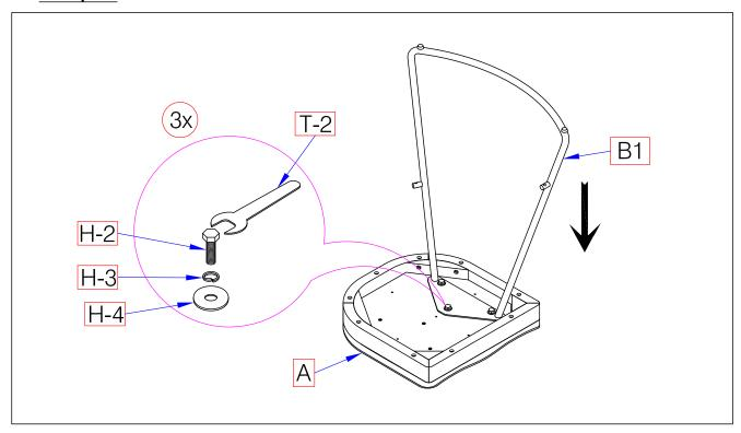
Place Seat Frame (A) on a non-marring surface. Position and secure Left Leg Frame (B1) to Seat Frame (A) with Flat Washers (H-4), Lock Washers (H-3) and Bolts (H-2) by using Wrench (T-2). Do not fully tighten Bolts.
