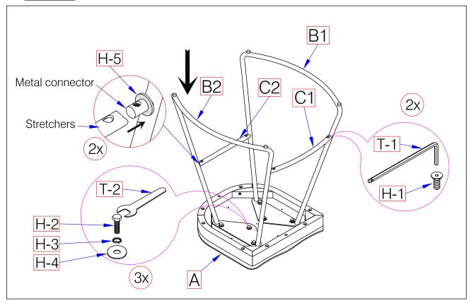
Attach Rubber Washers (H-5) to metal connectors on the Right Leg Frame (B2), then position and secure Right Leg Frame (B2) to assembled unit with Flat Washers (H-4), Lock Washers (H-3), Bolts (H-2) and Allen Bolts - Y Head (H-1) by using Wrench (T-2) and Allen Key (T-1). Fully tighten all Bolts and Allen Bolts - Y Head, as well as from all previous steps.
