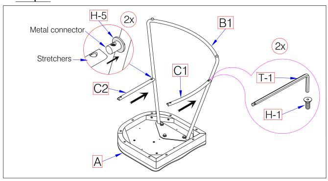
Attach Rubber Washers (H-5) to metal connectors on the Left Leg Frame (B1), then position and secure Front Stretcher (C1) and Back Stretcher (C2) to metal connectors on Left Leg Frame (B1) with Allen Bolts - Y Head (H-1) by using Allen Key (T-1). Do not fully tighten Allen Bolts - Y Head.
