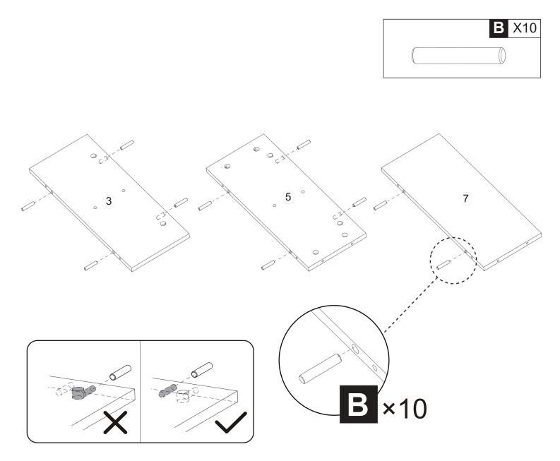
Attach Wooden Pin (B)\*10 to Board (3), (5) and (7).
