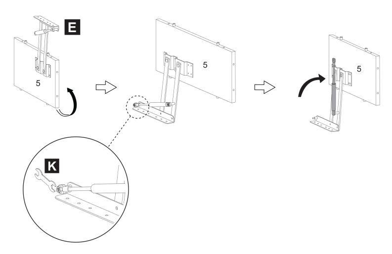
With Right Lifter **(E)** facing down, use Wrench **(K)** to unscrew the nut at the connection, then lift the damping rod.
