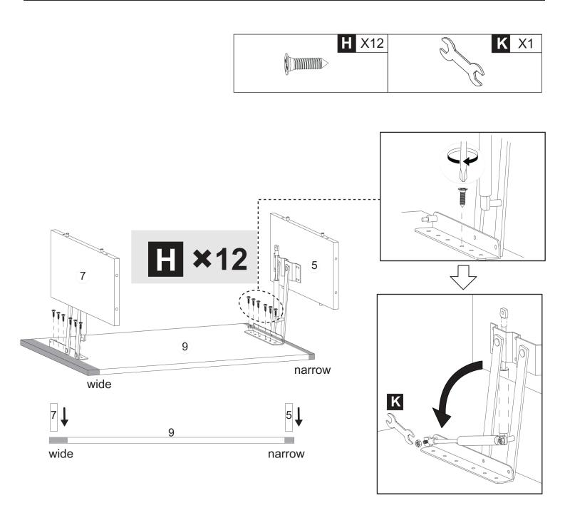
Using Bolts **(H)\*12**, install Left Lifter **(D)** to the "wide" side of Board **(9)** and Right Lifter **(E)** to the "narrow" side of Board **(9)**, then lower the damping rod and re-tighten the nut with Wrench **(K)**.
