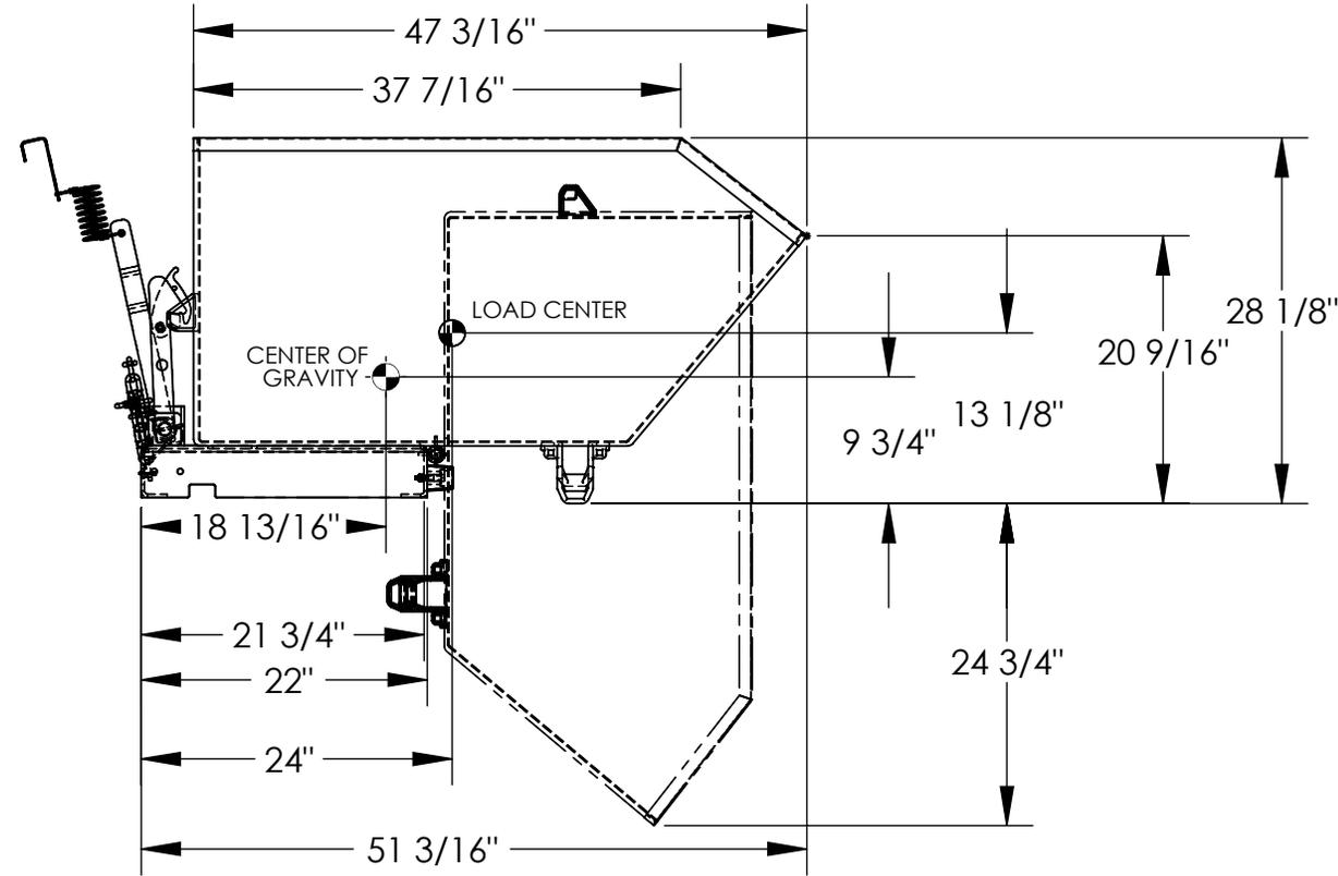
NEVER EXCEED LOAD CENTER RATING PER FORK TRUCK MANUFACTURER'S GUIDELINES. DO NOT USE THIS FORK TRUCK ATTACHMENT IF LOAD WILL EXCEED FORK TRUCK MANUFACTURER'S LOAD CENTER RATING.
