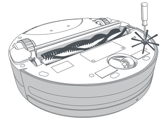
2. Secure Bob's side brush into the socket using the flat head screwdriver and screw.
