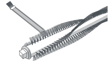
2. Clean the brush and the brush compartment from end to end using Bob's cleaning tool.
