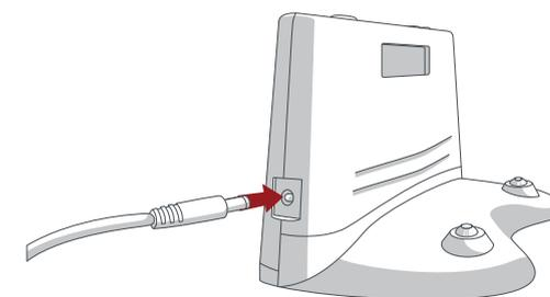
1. Plug the power adapter into the side of the charging station.
