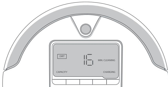
The words DIRT, MIN. CLEANING, CAPACITY, and CHARGING should be lit.
