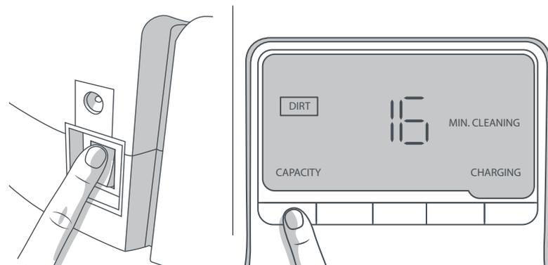
2. While holding down the UV button on Bob's cover, flip Bob's power switch ON.
