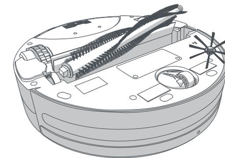
3. When done, replace the brush cap and insert the square end of the brush into the square notch inside Bob. Lastly, replace the screw.
