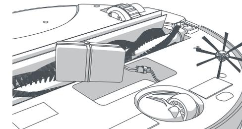
3. Slide the new battery into the compartment and replace the screws on the battery cover.
