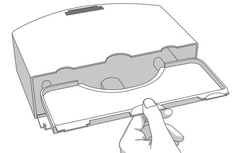
2. Pull out the filter frame from the roof of the dustbin.
