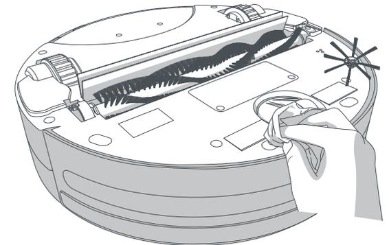
1. Wipe the wall and edge sensors using a soft cloth slightly dampened with cold water or alcohol.
