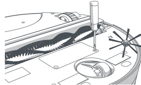
1. Remove the 2 screws on the battery cover using a Phillips head screwdriver.
