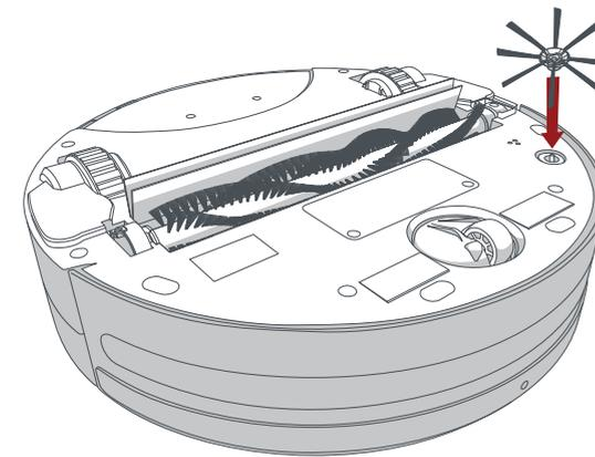
1. Flip Bob over onto a flat surface. Place the side brush over the empty socket on Bob's underside.
