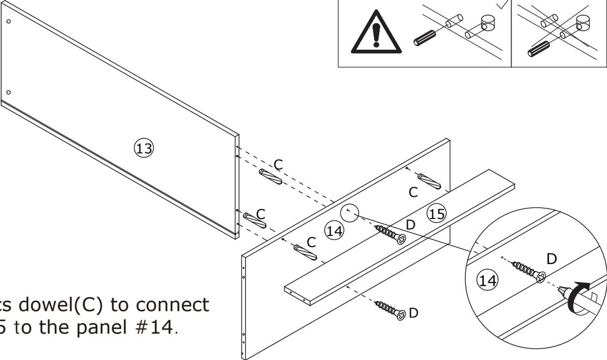
Using 2pcs dowel(C) to connect panel #15 to the panel #14.
