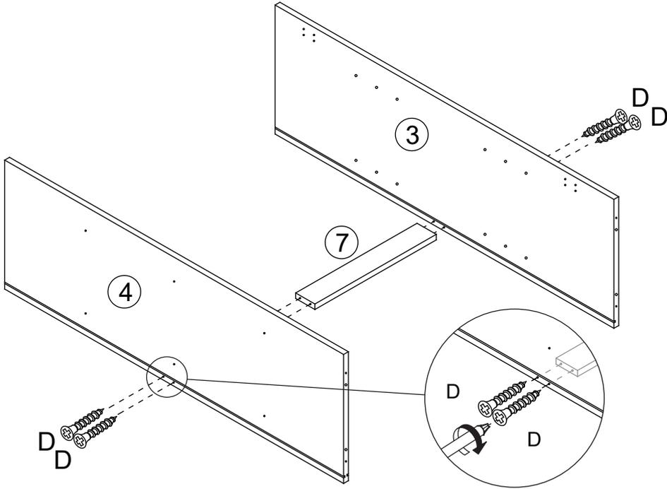
Using 4pcs screw(D) to connect panel #7 with panel #4 and #3 as shown.
