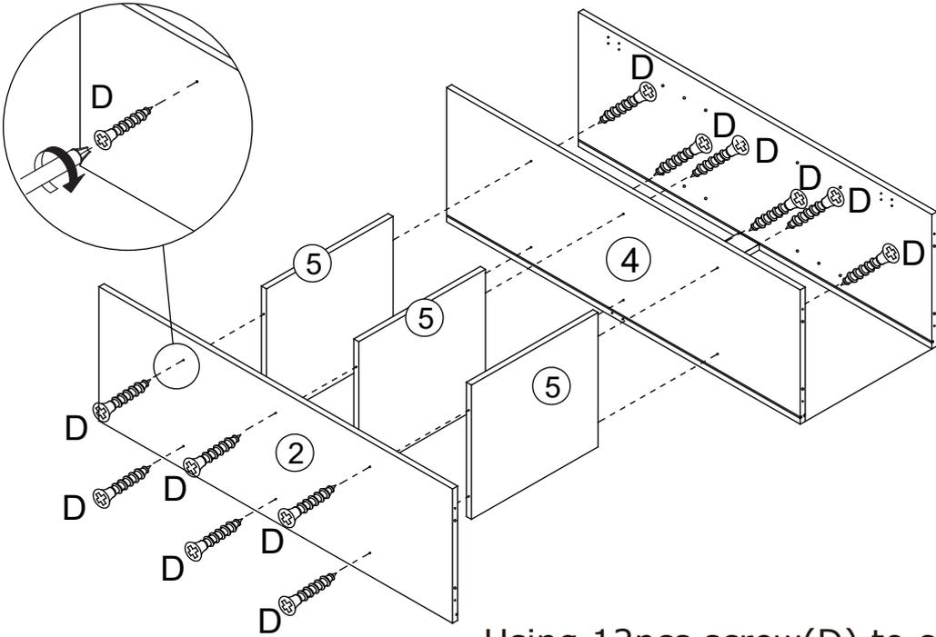
Using 12pcs screw(D) to connect 3pcs panel #5 with panel #4 and #2 as shown.
