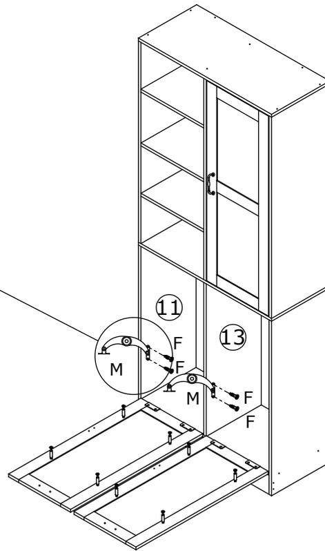
Using 4pcs screw(F) to lock the 2pcs flip(M) to the cabinet as shown.
