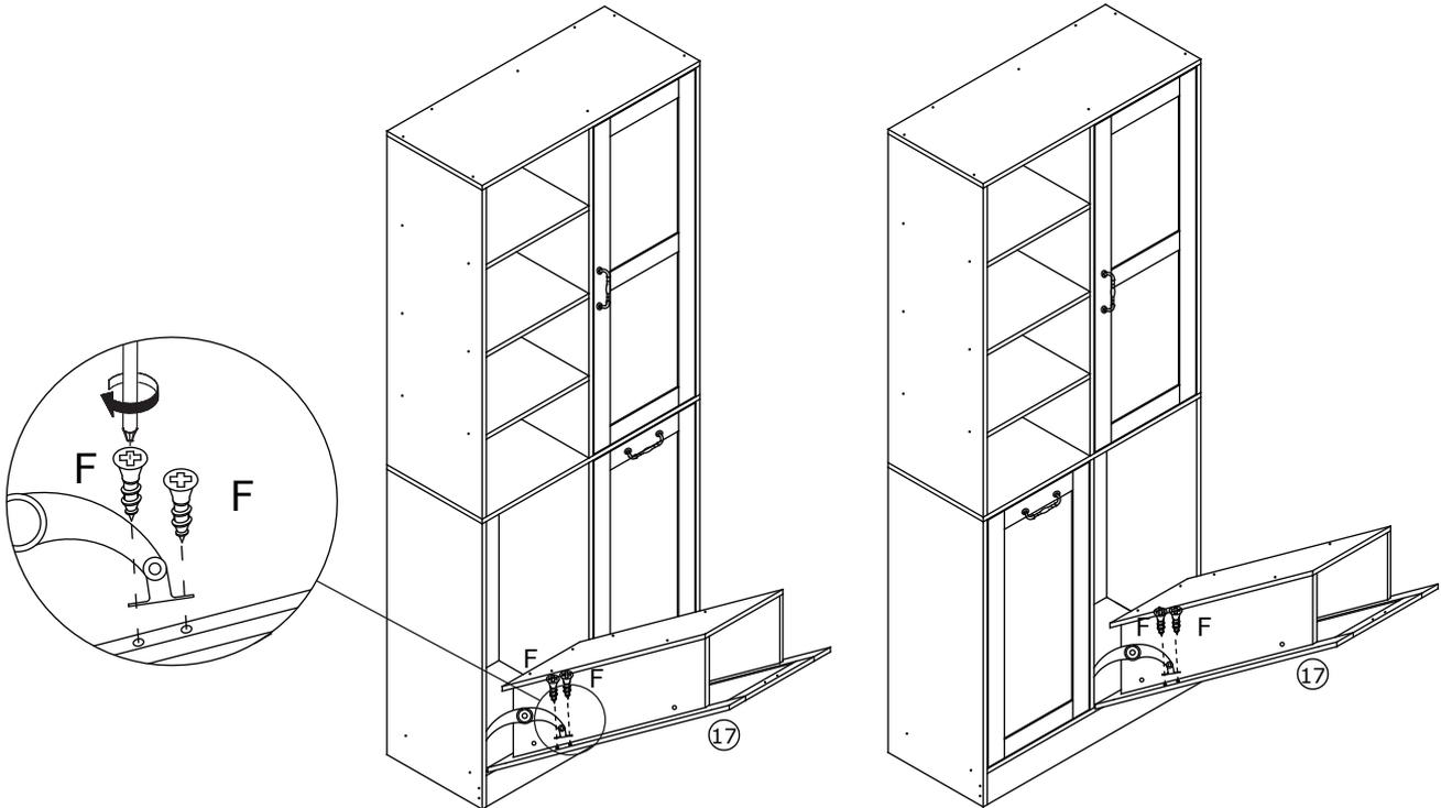
Using 4pcs screw(F) to lock the flaps to the door panel #17 as shown.
