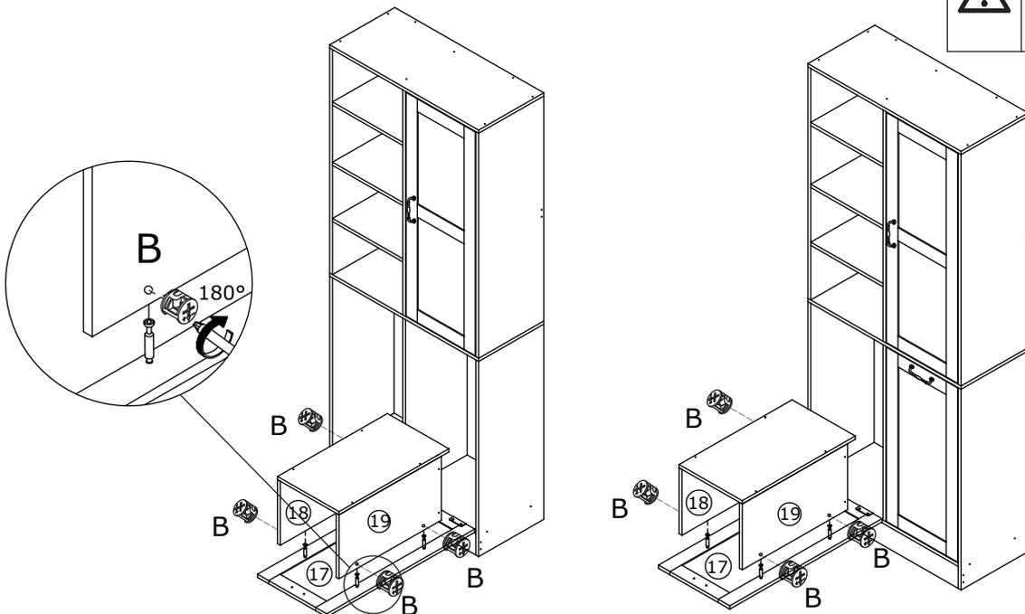
Connect panel #18,#19 to the door panel #17, insert cam lock(B) into panel #18,#19 as shown.
