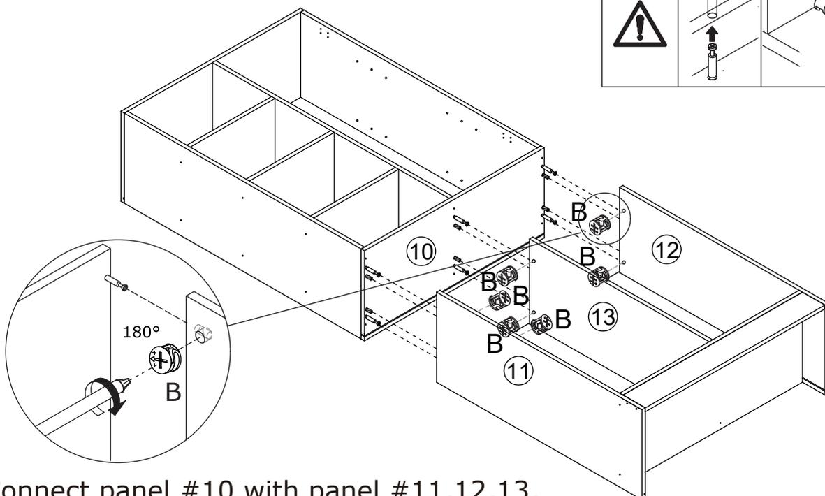
Connect panel #10 with panel #11, #12, #13, insert cam lock (B) into panel #11, #12, #13 as shown.
