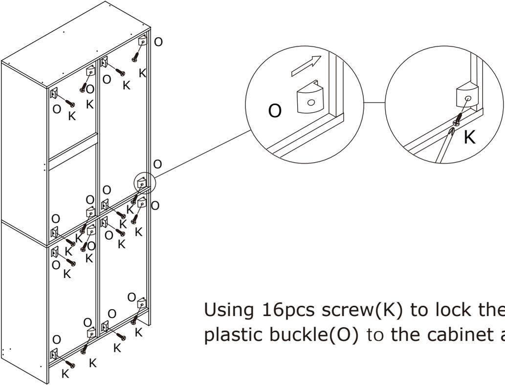
Using 16pcs screw(K) to lock the 16pcs plastic buckle(O) to the cabinet as shown.
