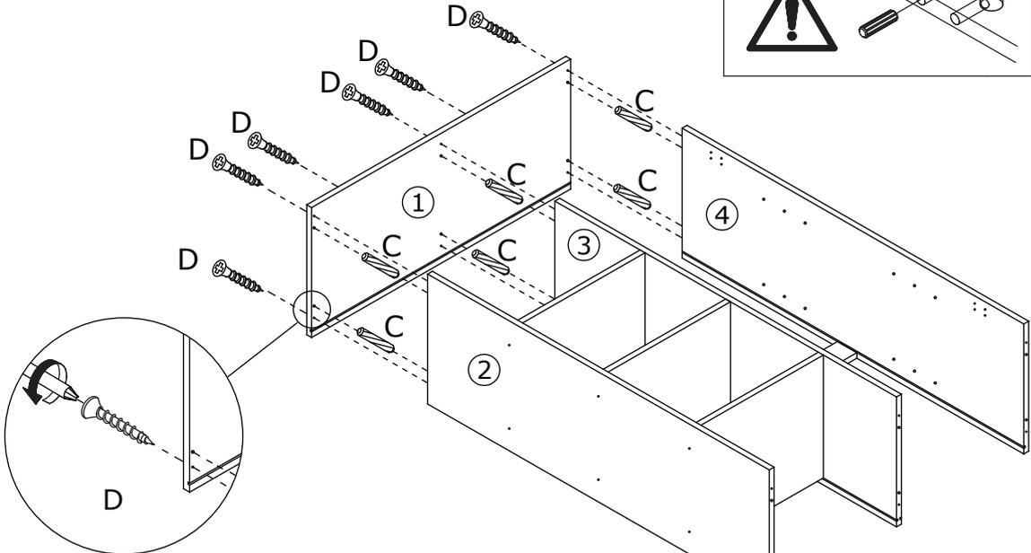
Using 6pcs screw(D) and 6pcs dowel(C) to connect panel #1 with panel #2,#3,#4 as shown.
