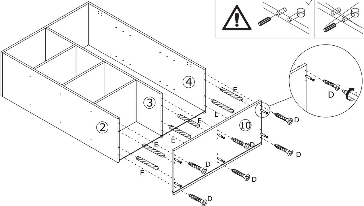
Using 6pcs screw(D) and 6pcs dowel(E) to connect panel #10 with panel #2,#3,#4 as shown.
