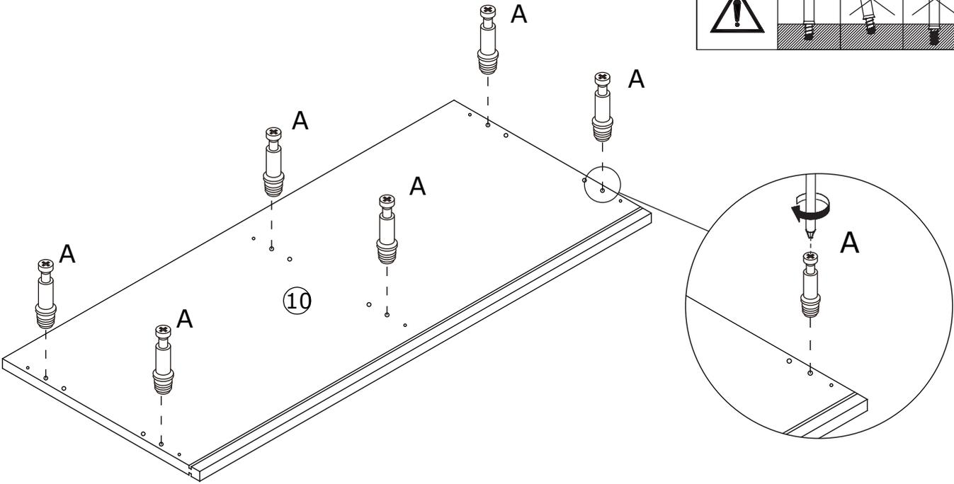
Insert 6pcs cam bolt(A) to panel #10 as shown.
