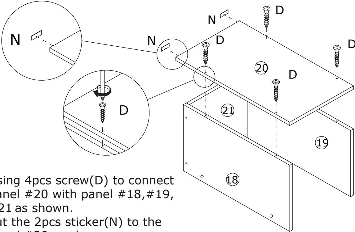
Using 4pcs screw(D) to connect panel #20 with panel #18,#19, #21 as shown.
