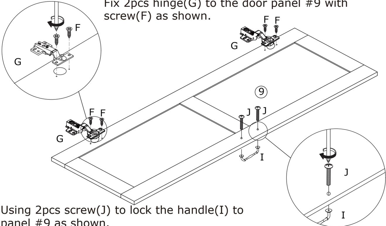
Using 2pcs screw(J) to lock the handle(I) to panel #9 as shown.
