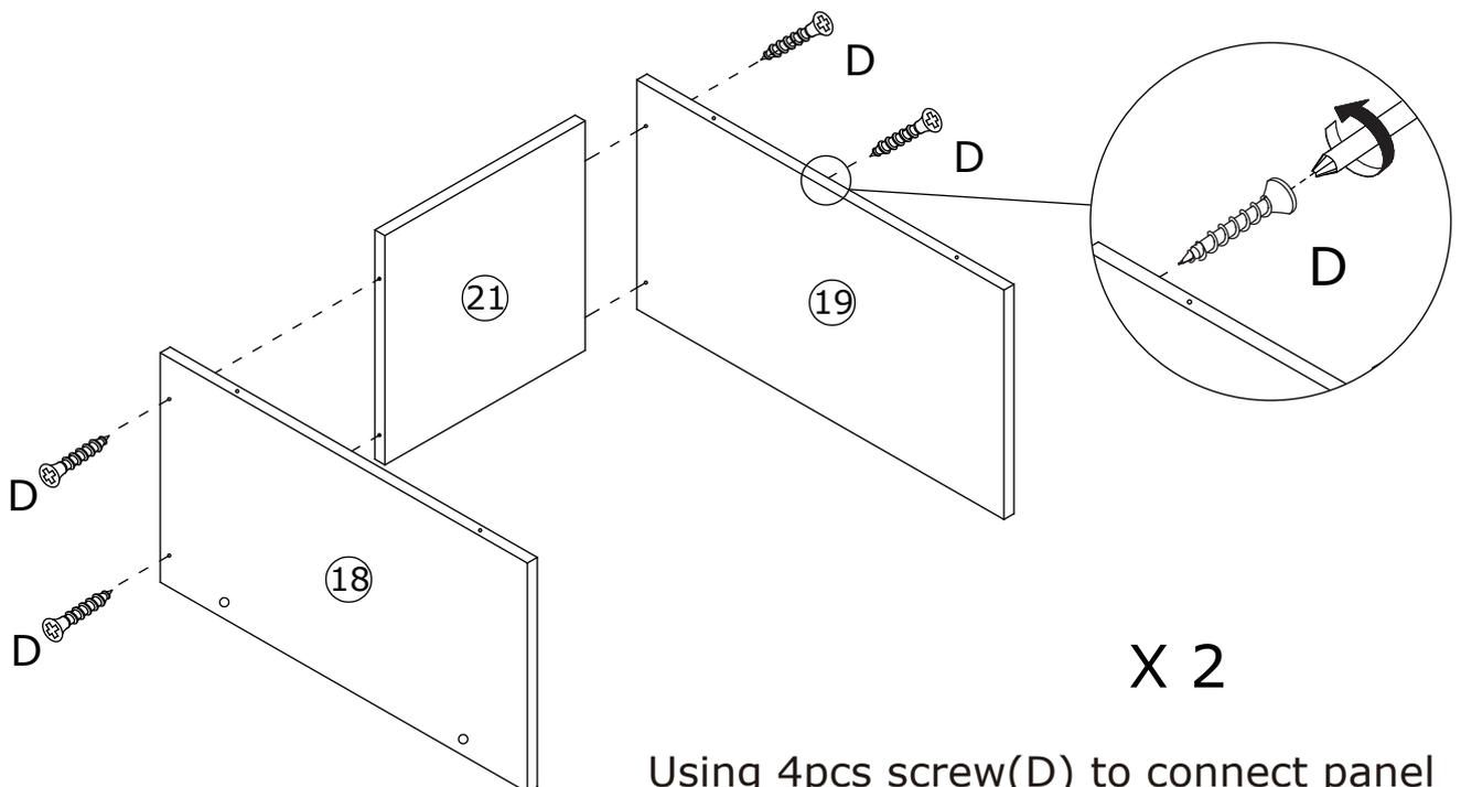
Using 4pcs screw(D) to connect panel #18,19 with panel #21 as shown.
