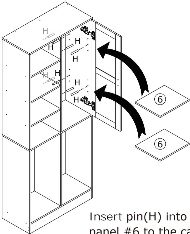
Insert pin(H) into the cabinet and put the shelf panel #6 to the cabinet as shown.
