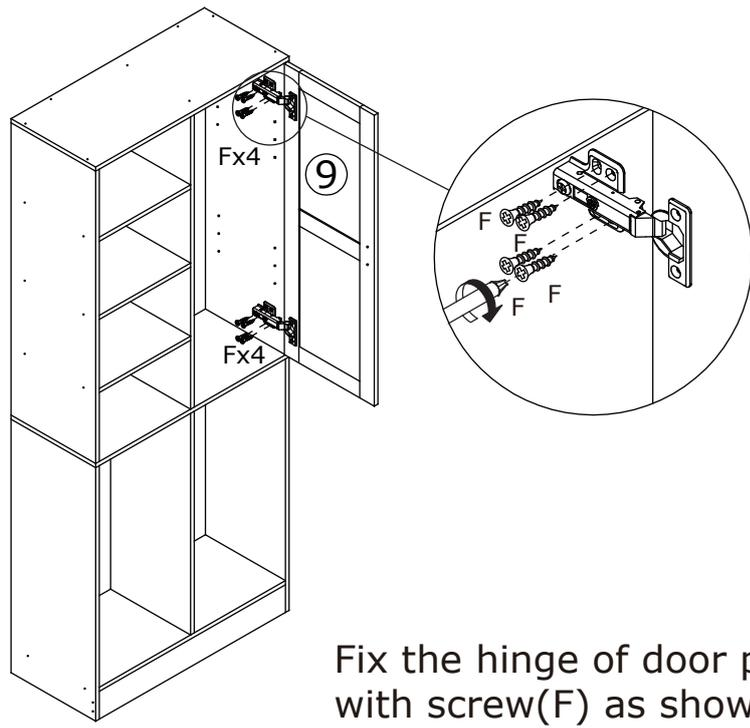
Fix the hinge of door panel #9 to cabinet with screw(F) as shown.
