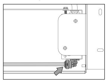
b. If the filter is installed in a remote location, attach an installer supplied length of 1/4 inch tubing to the 1/4 inch tubing from the water dispenser using a union coupling. The type of 1/4 inch tubing, copper or plastic, should meet all local regulations and building codes. This line should be insulated to prevent condensation.
