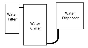
**Note:** The remote chiller can take from 24 to 48 hours to provide completely chilled water. Water lines must be insulated to prevent condensation.
