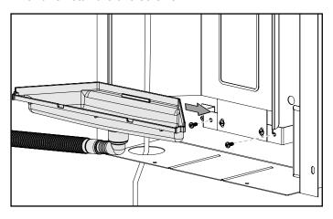
8. Route the drain hose through the filter box and attach the other end to the p-trap drain adapter using a hose clamp. The drain adapter is designed to be glued into a 1-1/4 inch PVC pipe.
