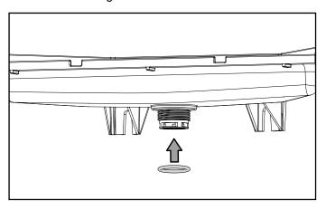
Thread the strainer into the drain adapter.
