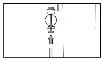
4. Connect a 1/4 inch insulated water line, copper or plastic, to the outlet connector of the filter.
