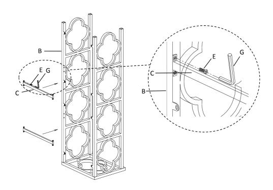
Attach frame(A) to frame(B) with allen wrench(G) to bolts(E), but not too tight. Fasten all bolts(E) tightly.
