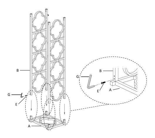
2 Attach stretcher(C) to frame (B) with allen wrench(G) to bolts(E), but not too tight.
