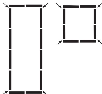
Side panels must be aligned **BEHIND** the gate and back panels to achieve the correct width. Be sure the 1.5" extended legs are positioned to be on the bottom.
