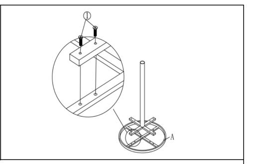
Attach the Table Top(A) to the Mounting Cross(B) and Table Leg(C) using Hardware(1) with Allen Key(2) as shown in Picture. Fully tighten at this stage.
