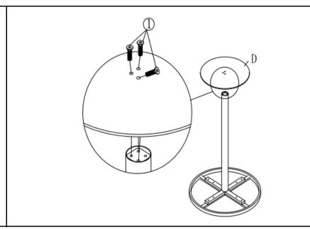
Attach the Base panel (D) to the Table Leg(C) using Hardware(1) with Allen Key(2) as shown in Picture.
