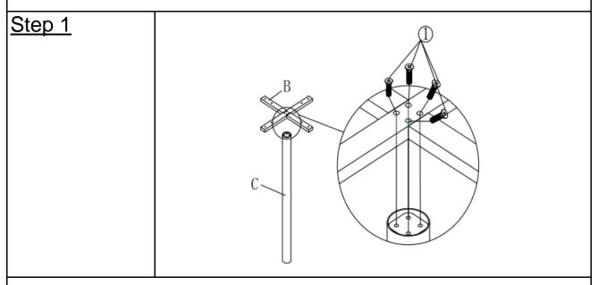
Open the carton and place all the parts onto a clean, non-marring surface. Attach the Mounting Cross(B) to Table Leg(C)using Hardware(1) with Allen Key(2) as shown in Picture .
