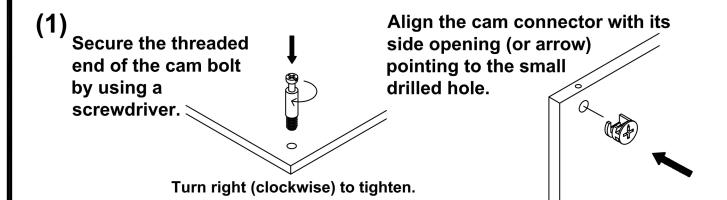
Insert the cam lock bolt into the pre-drilled hole above the cam
