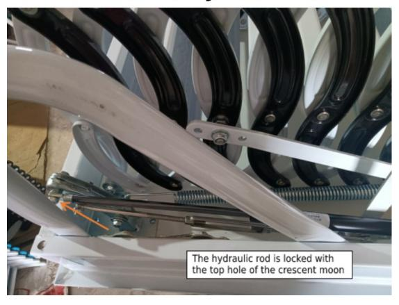
5.Insert the pry bar into the middle of the crescent and the frame, move the crescent upward and insert the screw hole into the second fulcrum hole under the crescent and lock the nut with the fixing screw, and the installation is completed.
