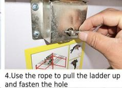
2.Lock the lever with the pin
