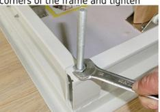
5.Screw on the triangle plate and tighten the nut
