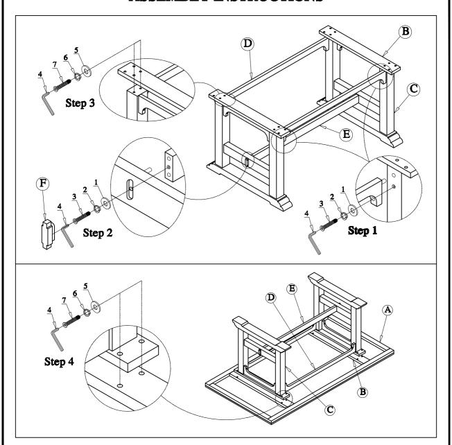
Step 1: Place Table side frames (C), on the floor. Attach Side Stretcher (D) to the Table side frames (C) by inserting Small Flat Washer (1), Small Spring Washer (2), and Small Bolt (3). Tighten with Allen Key (4)
