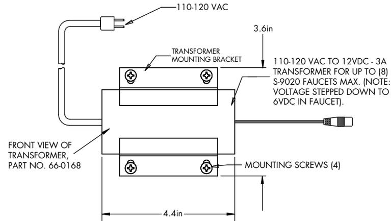
NOTE: MOLDED PLUGGABLE CONNECTION. WHERE ELECTRICAL CODES CALL FOR HARDWIRE, CUT OFF PLUG AND HARDWIRE PER ELECTRICAL CODE(S).
