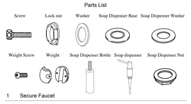
Place faucet on sink by feeding hoses down through the center hole in sink. Remove the mounting nut and nylon washer from threaded collar. Note that the black rubber gasket at the base of the faucet body remains in place as used to create a seal after faucet is installed.
