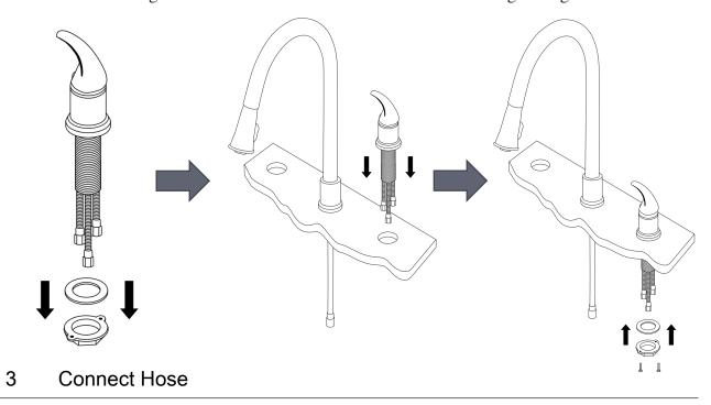
Connect sprayer hose. Attach the weight to the hose at a length suitable to you (The further from the end you place the weight the longer your reach will be when pulling the hose out for use). You may move the weight to adjust the pull-out length of the hose. Carefully tighten the weight.
