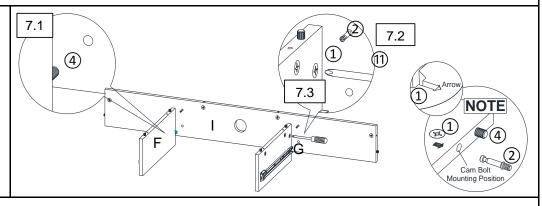
**7.1)** Insert Positioning Dowels(④) from Left Center Panel(F) and Right Center Panel(G) into mounting positions on Back Panel(I).
