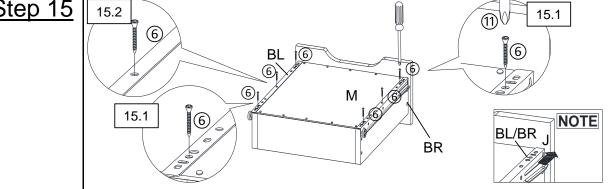
15.1) Attach Drawer Left Bottom Rail(BL) and Drawer Right Bottom Rail(BR) to Drawer Bottom Panel(M) using Screws(6) with Screwdriver(11) where indicated.
