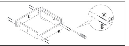
Attach Drawer Side Panels(K) to Drawer Front Panel(J) and Drawer Back Panel(L) using Screws(®) with Screwdriver(11).
