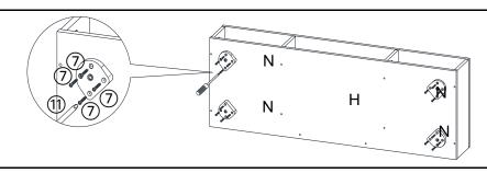
Attach Leg Supports(N) to Bottom Panel(H) using Screws(⑦) with Screwdriver(⑴).
