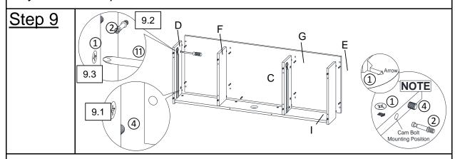
**9.1)** Insert Positioning Dowels(④) from Left Side Panel(D), Right Side Panel(E), Left Center Panel(F) and Right Center Panel(G) into mounting positions on Top Panel(C).
