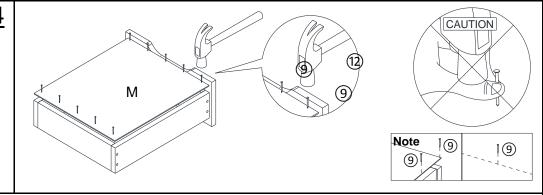
Attach Drawer Bottom Panel(M) to Drawer Assembly using Nails(9) with Hammer((12)).
