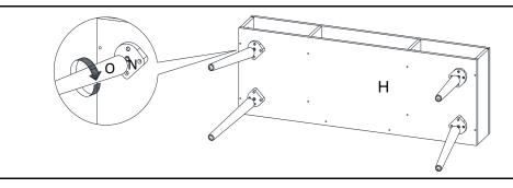
Attach Legs(O) to Leg Supports(N) by rotating the Legs clockwise by hand.
