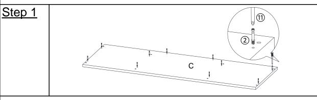
Unpack and place all parts on a clean, non-marring surface. Attach Cam Bolts(2) to mounting positions on Top Panel(C) with Screwdriver(11).
