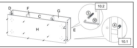
**10.1)** Insert Positioning Dowels(④) from Left Side Panel(D), Right Side Panel(E), Left Center Panel(F) and Right Center Panel(G) into mounting positions on Bottom Panel(H).
