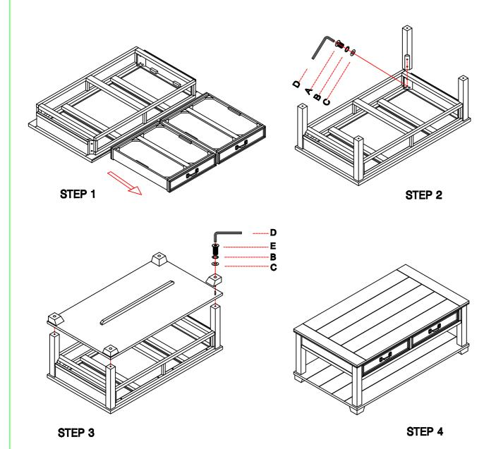
DO NOT TIGHTEN SCREWS UNTIL COMPLETELY ASSEMBLED
