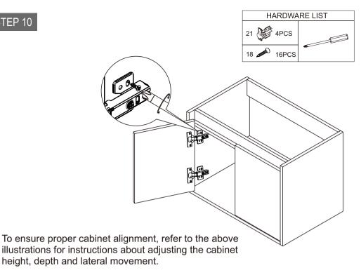
+2.5mm A.Depth adjustment +5mm B.Side to side adjustment
