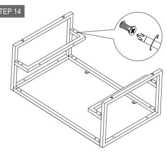
• Refer to the illustration, combine the iron frame and cabinet and lock it with screws.
