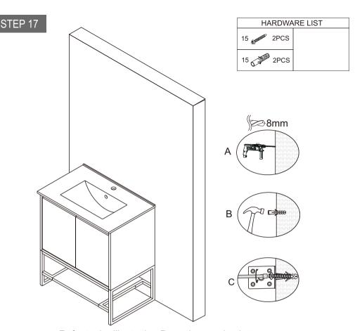
• Refer to the illustration, Draw the spacing between the walls on the cabinet, punch holes in the wall, and fix the cabinet to the wall with screws. Then tighten the nut cover.
