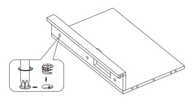
• Refer to the illustration, Then tighten the cam lock with the cover.
