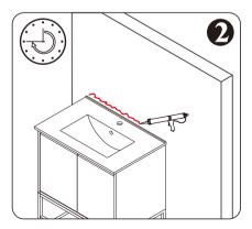
Install the basin on the cabinet with glue. Put into use after 24 hours.
