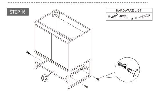
• Refer to the illustration, combine the iron frame and cabinet and lock it with screws.
