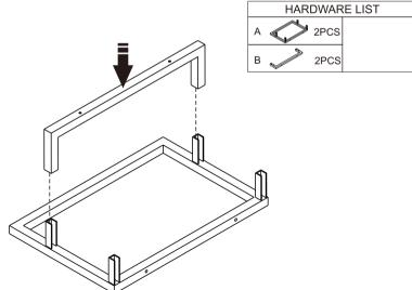
• Refer to the illustration, combine the iron frame and cabinet and lock it with screws.
