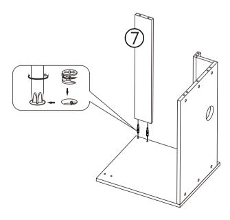
• Refer to the illustration, Then tighten the cam lock with the cover.
