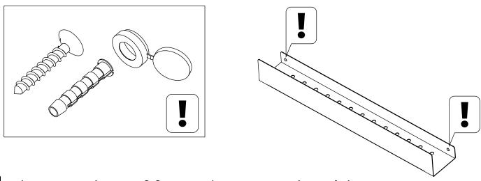
The number of fastening sets should correspond with the holes in the back of the shelf
