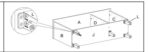
Attach Legs(L) to Bottom Panel(J) using Screws(6) with Screwdriver(3).
