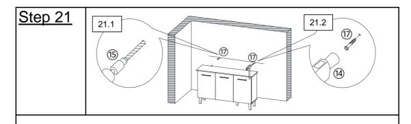
**21.1)** Drill two holes on wall at same height as Metal Brackets(16) on Shoe Cabinet with Power Drill(15).
