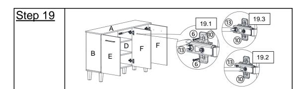
**19.1)** Attach Connectors(⑩) to Left Side Panel(B), Right Side Panel(C) and Center Panel(D) with Screws(⑥) using Screwdriver(③).
