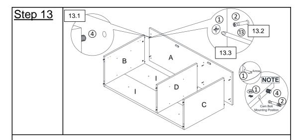
**13.1)** Insert Positioning Dowels(④) from Left Side Panel(B), Right Side Panel(C) and Center Panel(D) into mounting positions on Top Panel(A).
