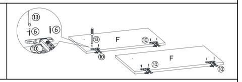
Attach Connectors(®) to Right Door Panels(F) using Screws(6) with Screwdriver(®).
