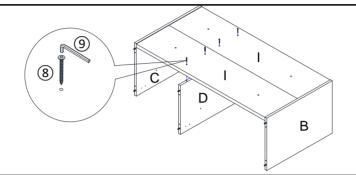
Attach Back Panel(I) to Shoe Cabinet Assembly using Cap Wood Screws(8) with Allen Key(9).
