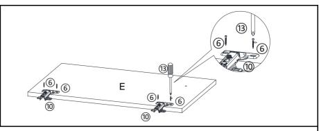
Attach Connectors(⑩) to Left Door Panel(E) using Screws(⑥) with Screwdriver(⑴).
