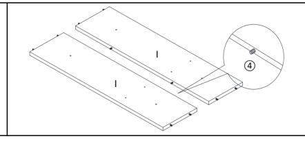
Attach Positioning Dowels(4) from Back Panel(I) into mounting positions on the other Back Panel(I).
