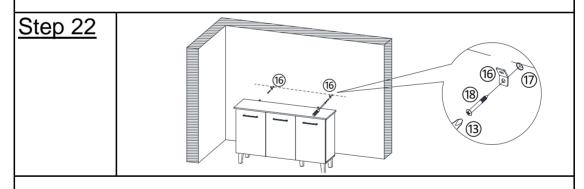
Attach Metal Brackets(16) to Wall Plugs(17) using Wall Plug Screws(18) with Screwdriver(13).
