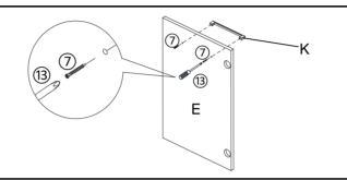
Attach Handle(K) to Left Door Panel(E) using Screws(⑦) with Screwdriver(③).
