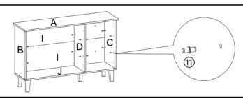
Insert Metal Shelf Supports(11) into mounting positions on Left Side Panel(B), Right Side Panel(C) and Center Panel(D) by hand.
