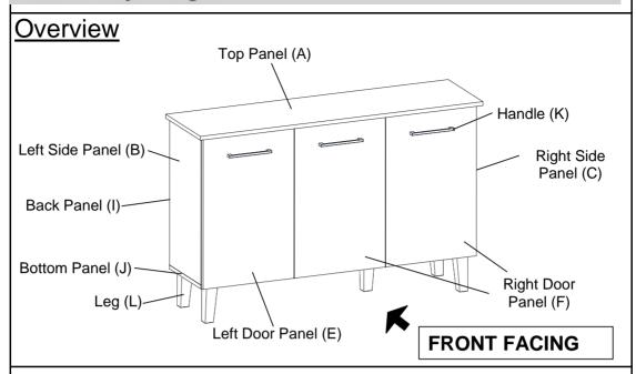
This Shoe Cabinet has multiple parts and may require up to 60 minutes to assemble. To give you an overview of the Shoe Cabinet parts, the above picture is to help you put the various parts into perspective. Please read through the instructions below to familiarise yourself with the parts and steps before assembly.
