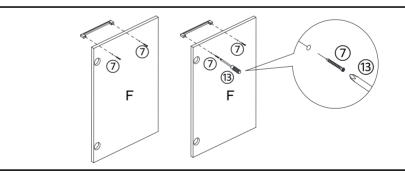
Attach Handles(K) to Right Door Panels(F) using Screws(⑦) with Screwdriver(⑥).
