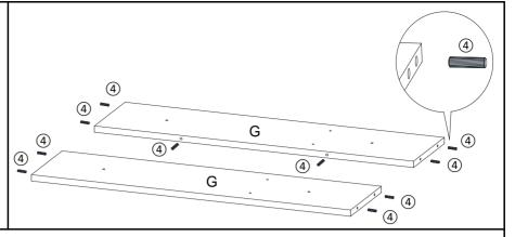
Insert Positioning Dowels(4) into mounting positions on Back Panel(G) by hand.
