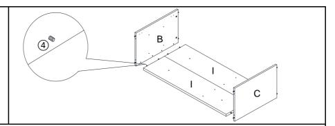
Insert Positioning Dowels(④) from Back Panel(I) into mounting positions on Left Side Panel(B) and Right Side Panel(C).
