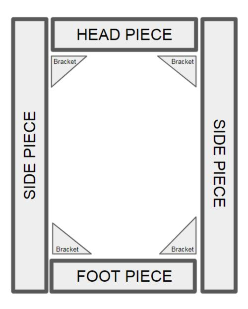
4. Stand the **Foot Piece** up on its side and place at the bottom of the two **Side Pieces**, ensuring the **Side Pieces** are on the <u>OUTSIDE</u> of the **Foot Piece**. The black vinyl should be facing the outside. Screw the **Foot Piece** to both **Side Pieces** using the **Large Corner Brackets** and the **Short Screws** to secure them together.
