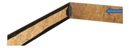
3. Stand the other **Side Piece** up on its side and ensure the black vinyl side is facing the outside. Line up the **Side Piece** to the other end of the **Head Piece** with the <u>INSIDE</u> edge of the side piece. Screw the **Large Bracket** into the inside corner of these 2 pieces using the **Short Screws** to secure them together.
