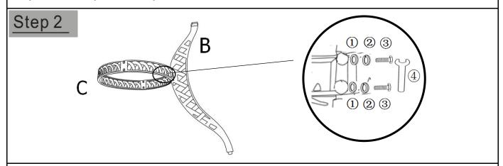
Loosely attach the Central Round Support Ring(C) to Table Leg(B) using Washers(1), Spring Washers(2), and Hex Bolts(3) with the Spanner(4).
