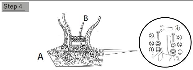
Lay the Table Top(A), top facedown, onto a flat, soft, clean surface. Loosely attach the Table Legs(B) to the the Table Top(A) using Washers(1), Spring Washers(2), and Hex Bolts(3) with the Spanner(4). **Do not fully tighten Bolts.**
