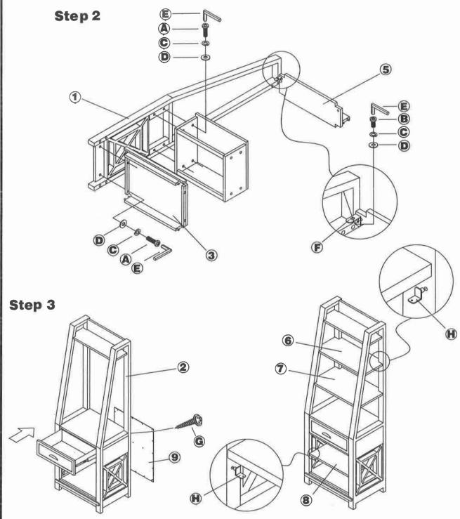
NOTE: DO NOT TIGHTEN ALL THE BOLTS UNTIL THEY ARE INSTALLED IN CORRESPONDING HOLES!
