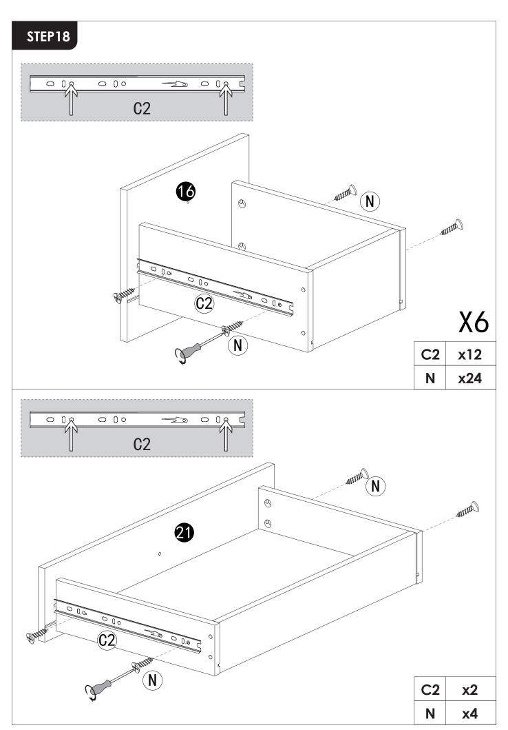
**REMARK:** Align the slide runners on the drawer with the unit and push it carefully inside until it stops.
